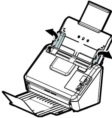
4. Load the stack of document **face down** with the top of the pages pointing into the feeder.
