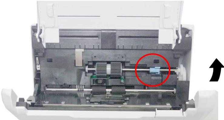
4. Detach the right end of the ADF roller from the scanner and remove the ADF roller.
