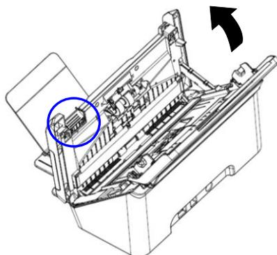
3. Refer to the subsequent section [7.4 Replacing the ADF Friction Roller](#) on how to remove the Friction Roller.
