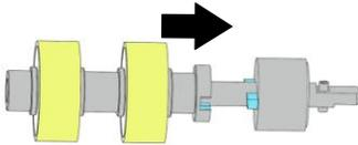
2. Insert the left end of the Friction Roller to the slot. Make sure the flat side is up as shown.
