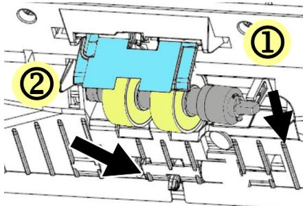
5. Remove the rollers from the shaft.
