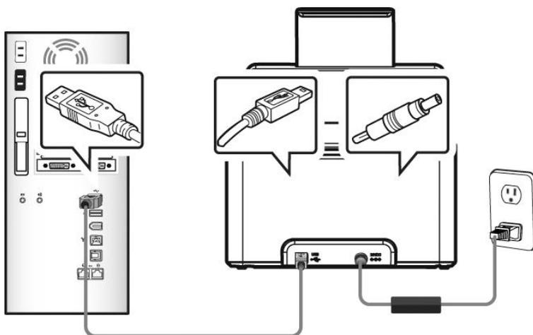
2. The computer should detect a new USB device and prompt a **"New Hardware Found"** message.
