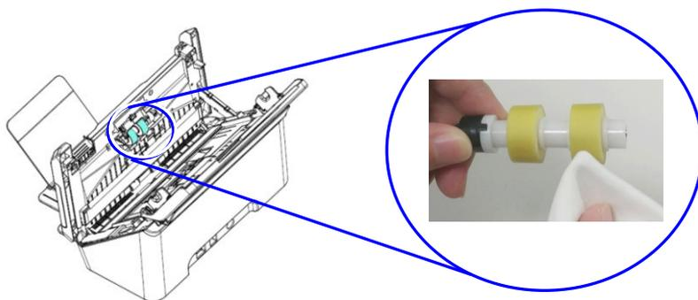
5. Refer to the subsequent section 7.4 Replacing the ADF Friction Roller on how to remove the Friction Roller.
