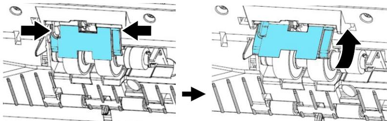
4. Press the right end of the Friction Roller externally to detach it from the slot and then detach the left end from its hole.
