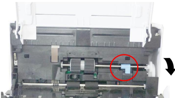
3. Close the ADF roller cover. A snap-in sound could be heard if correctly installed.
