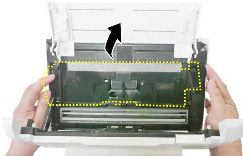
3. Move the tab of the ADF roller **UP** as indicated.
