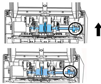
3. Close the ADF roller cover. A snap-in sound could be heard if correctly installed.
