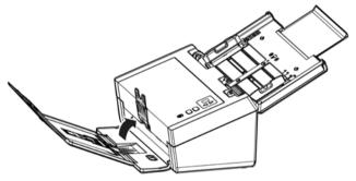
2. Slide the position adjuster of the output tray to make the output tray in a flat position.
