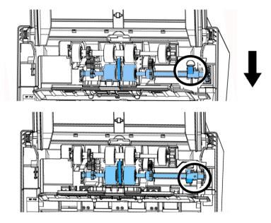
3. Move the tab of the ADF roller **DOWN** as indicated.
