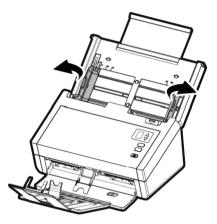
4. Load a stack of document face down with the top of the pages pointing into the feeder.
