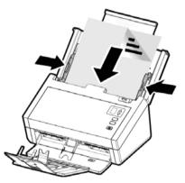
5. Verify that the paper guides are aligned with the edges of the stack.
