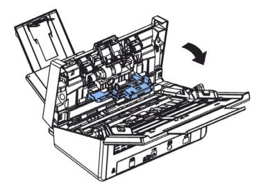
4. Press the right end of the reverse roller externally to detach it from the slot and then detach the left end from its hole.
