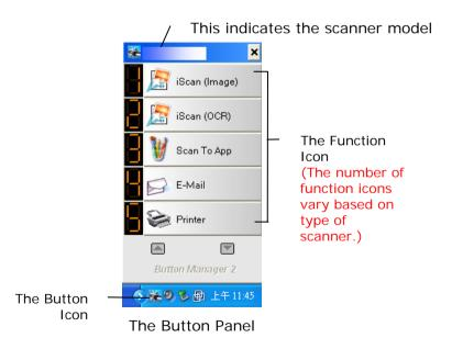
The Button Panel shows the first five scanning buttons. Right-click the button (function) you wish to check. The Button Properties window appears.
