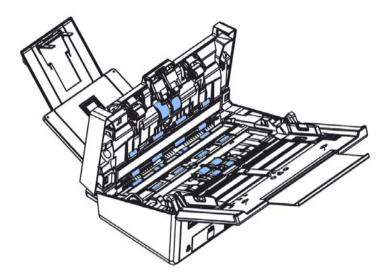
4. Press both sides of the cover of the ADF reverse roller and pull the cover down.
