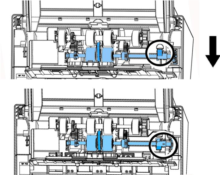
4. Detach the right end of the ADF roller from the slot and remove the ADF roller.
