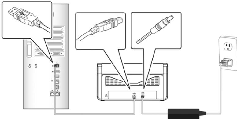
2. The computer should detect a new USB device and prompt a **"New Hardware Found"** message.
