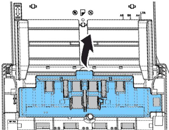
3. Move the tab of the ADF roller **DOWN** as indicated.
