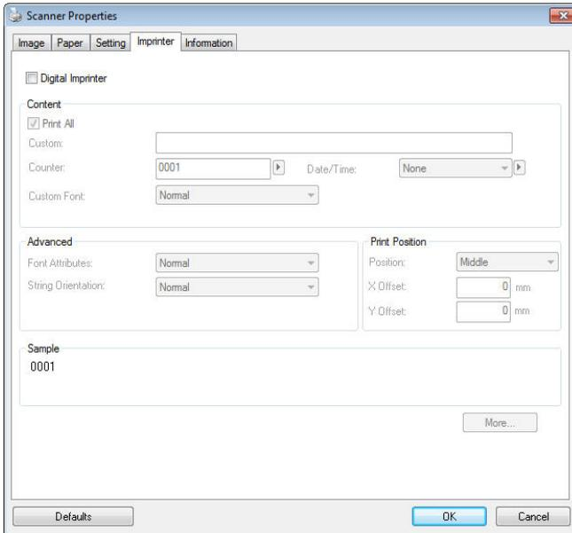
**Choice: External Imprinter, Digital Imprinter.** If you have installed an external imprinter, choose external imprinter. If you do not have an imprinter, choose digital imprinter. Note External Imprinter provides a vertical and rear-side print capability while digital printer provides a horizontal and front-side print capability.
