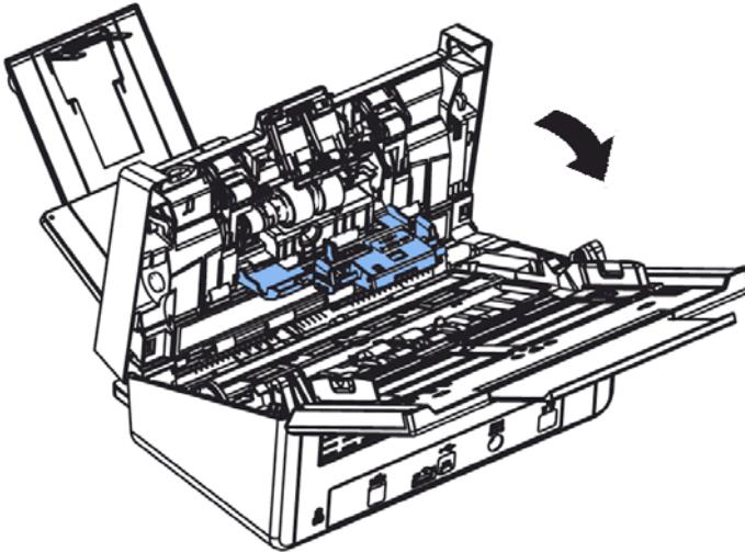
4. Press the right end of the reverse roller externally to detach it from the slot and then detach the left end from its hole.
