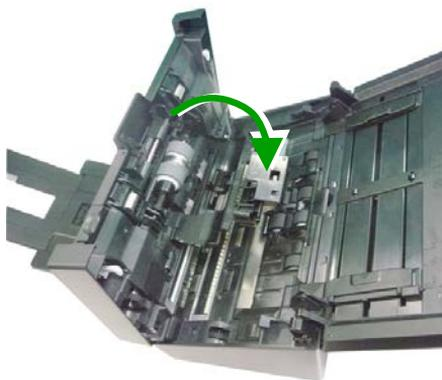
4. Press the right end of the reverse roller externally to detach it from the slot and then detach the left end from its hole.
