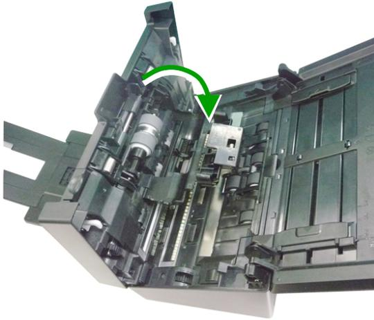
5. Press and wipe the rollers one by one. Rotate the roller until the surfaces are completely cleaned.
