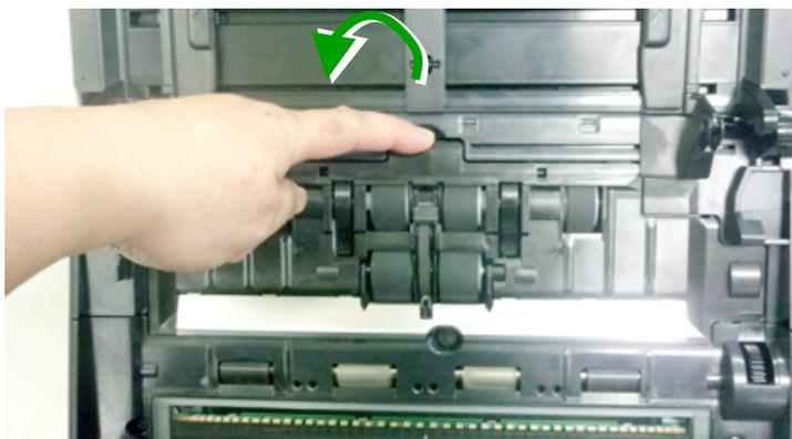
3. Move the tab of the ADF roller **DOWN** as indicated.
