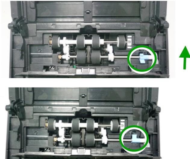
3. Close the ADF roller cover. A snap-in sound could be heard if correctly installed.
