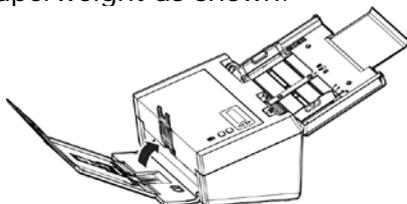
2. Slide the position adjuster of the output tray to make the output tray in a flat position.
