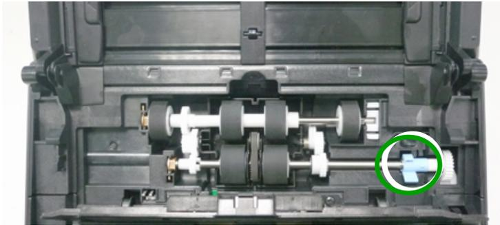
4. Detach the right end of the ADF roller from the scanner and remove the ADF roller.
