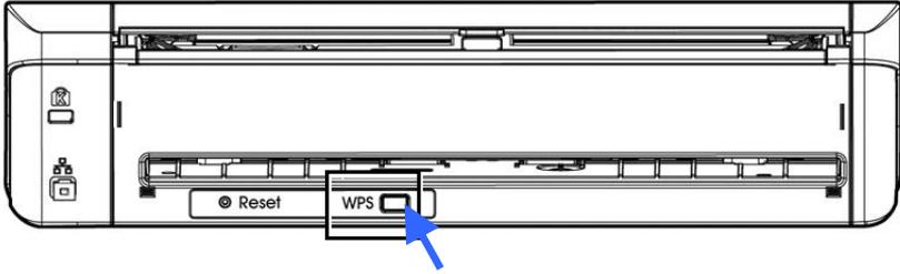
5. If the connection is successful, the Wi-Fi LED light of the scanner will be flashing. (Refer to the user's guide of your access point for the connection result.)
