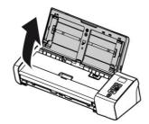
2. Press the ADF Release button to open the feeder cover.
