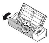
3. Wipe the separation pad, rollers and the glass with the cleaning cloth.
