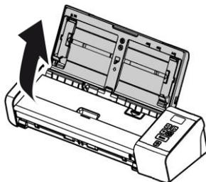
2. Press the ADF Release button to open the feeder cover.
