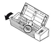
3. Press two arms of the separation pad inwardly with two fingers (0) and lift it up (2) to remove the separation pad.
