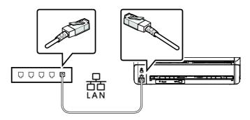
2. Press the Wi-Fi button on the control panel to enable the Ethernet function. (The Wi-Fi button is designed to enable both the Wi-Fi and Ethernet function.)
