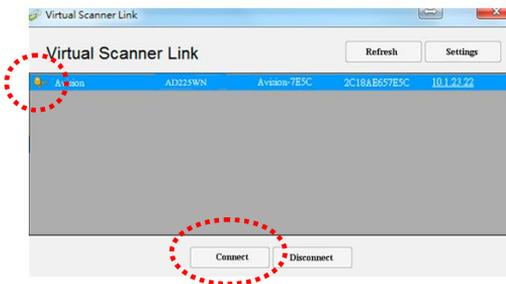
3. After the scanner has been connected successfully, launch your TWAIN-compliant image-editing software application to start a scan.
