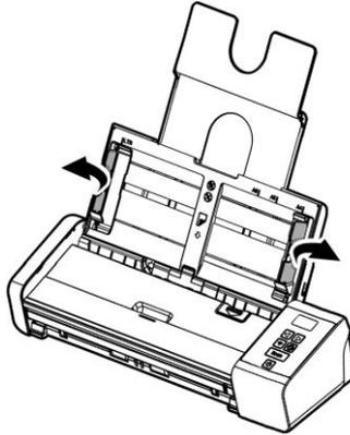
3. Load the stack of document **Facing Down** with the top of the pages pointing into the feeder.
