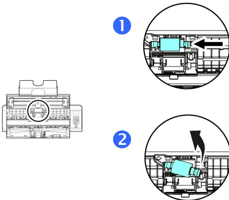
6. Attach the new feed rollers. Insert the left end of the shaft to the notch and slide the feed roller to the right. A snap-in sound could be heard.
