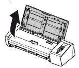
2. Press the ADF Release button to open the feeder cover.
