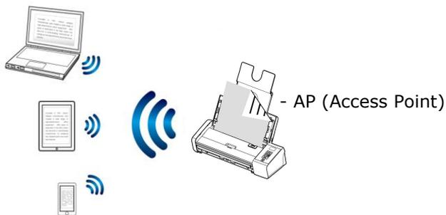
1. Press the Wi-Fi button to turn on Wi-Fi. If the connection is successful, the blue Wi-Fi LED light will be flashing.
