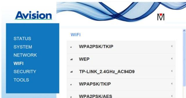
2. Choose the network name (SSID) which you wish to connect to and then click the [**Connect**] button. (Wait for 60 seconds while the connection is processed.) If required, type your network password (or security key) and click [**OK**].
