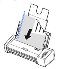
4. Verify that the paper guides are aligned with the edges of the stack.
