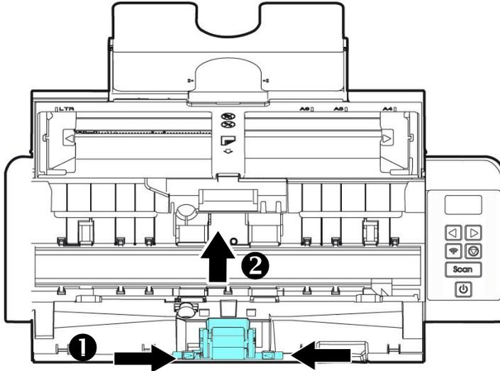
4. Hold two arms of the separation pad with two fingers and attach the new separation pad to the scanner.
