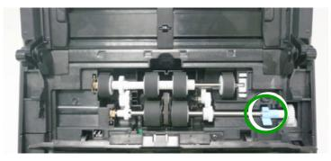
4. Detach the right end of the ADF roller from the scanner and remove the ADF roller.
