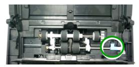
3. Close the ADF roller cover. A snap-in sound could be heard if correctly installed.
