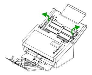
4. Load the stack of document face down with the top of the pages pointing into the feeder.
