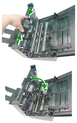
4. Press the right end of the reverse roller externally to detach it from the slot and then detach the left end from its hole.
