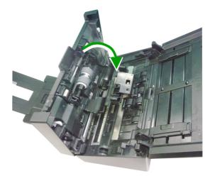
5. Press and wipe the rollers one by one. Rotate the roller until the surfaces are completely cleaned.
