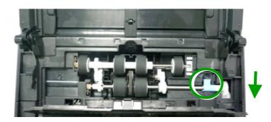
3. Move the tab of the ADF roller **DOWN** as indicated.
