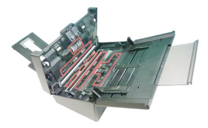
4. Press both sides of the cover of the ADF reverse roller and pull the cover down.
