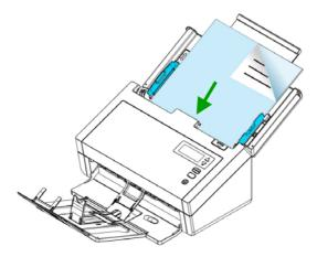
5. Verify that the paper guides are aligned with the edges of the stack.
