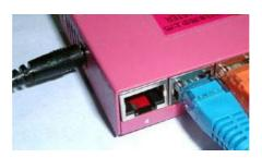
2. Connect the other end to the LAN port marked  $\Box \Box$  at the back of the product as shown.
