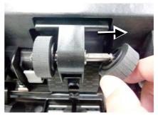
**3.** Press down the hook next to the left roller to remove the left roller.
