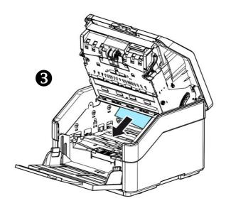
3. Close the ADF by pressing down on the center of the ADF to return it to its original position until it clicks into place.
