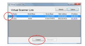
3. After the scanner has been connected successfully, launch your TWAIN-compliant image-editing software application to start a scan (Figure A).
