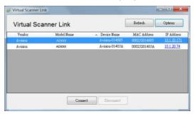
Choose the scanner you wish to connect and then press [Connect]. If connection is successful, a connection mark will be displayed as shown.
