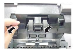
3. Press down the hook next to the right roller to remove the right roller.
