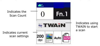
Refer to chapter 4 – <u>Using Avision Properties Dialog Box</u> on how to start a scan with TWAIN user interface.
