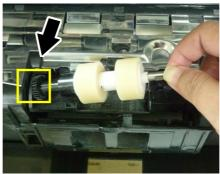
5. Insert the right end of the new Reverse Roller to its slot. If successful, a crispy snap-in sound can be heard.
