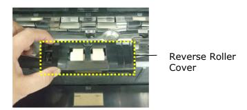
3. Place your fingers in the center of the Reverse Roller Assembly and lift it up to remove it from the slot.
