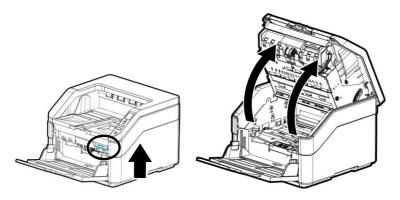
2. Carefully pull the paper out of the ADF unit.
