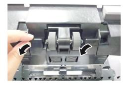
3. Pull down the tab to remove the ADF roller.
