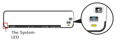
2. The **System LED** will be first lit in red and then lit in green steadily. This indicates the scanner is in ready status.
