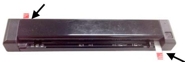
**Remove the protective tapes from the scanner.**
