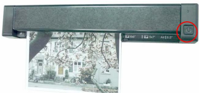
Align the document Face Up to the left edge of the feeder. All images are scanned in color mode.
