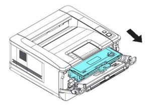
**4.** Remove the toner cartridge from the drum unit as shown.
