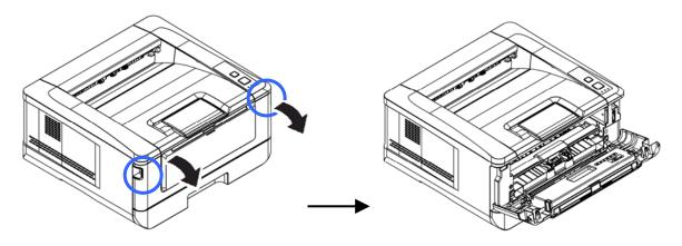
**5.** Lift the handle of the drum unit up and then pull it out as shown.
