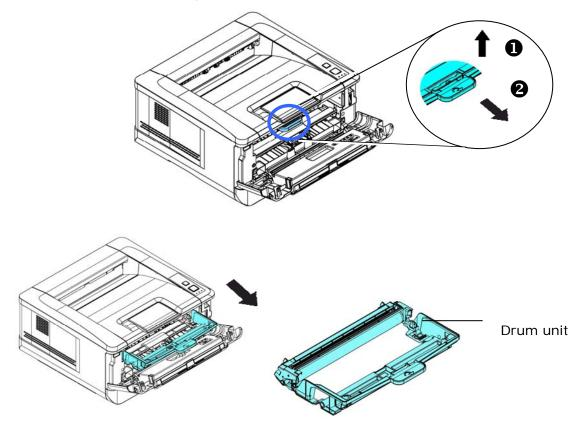
**2.** Lift the handle of the drum unit and toner cartridge assembly and gently remove the assembly.
