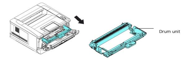
**3.** Remove the toner cartridge from the drum unit as shown.
