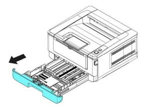
**3.** Lift the handle of the main paper tray and then pull out the main tray.
