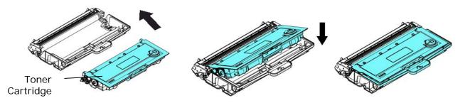
**5.** Hold the handle of the drum and toner cartridge assembly and insert the assembly to its original place.
