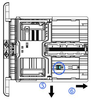
To move the tray back to the original A4 length, press down the second length adjustment latch ( $\bigcirc$ ), and at the same time slide the manual tray to the left (8).
