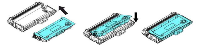
2. Hold the handle of the toner cartridge and insert the toner cartridge to its original place. Press the handle to fix it firmly in place.
