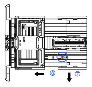
7. Load the paper stack with the **Printing Side Facing Down** as illustrated.
