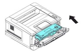
**6.** Press down the handle of the toner cartridge to fix the toner cartridge.
