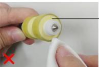
Do not let the cloth moisturized with alcohol touch the foam beneath the surface of the roller or let the excessive alcohol flow into the foam.
