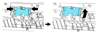
4. Press the right end of the Friction Roller externally to detach it from the slot and then detach the left end from its hole.
