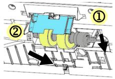
5. Remove the rollers from the shaft.
