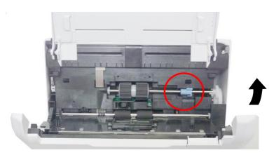
4. Detach the right end of the ADF roller from the scanner and remove the ADF roller.
