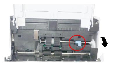
3. Close the ADF roller cover. A snap-in sound could be heard if correctly installed.
