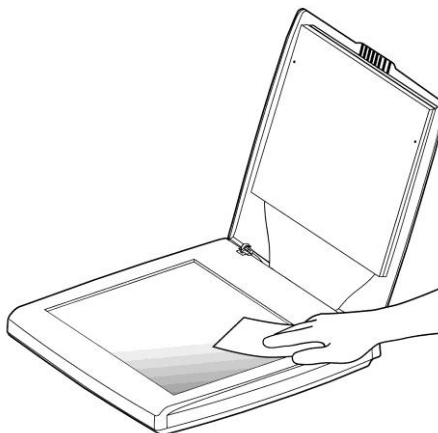
Figure 5-1 The cleaning area
