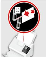
An illustration of a white scanner with a red circle and a white 'X' over it, indicating a paper jam. Red arrows point to the paper path. | <p>Falhou ao pegar o papel</p>                | <ol style="list-style-type: none"><li>1. Ventile os documentos.</li><li>2. Coloque o documento com as bordas levemente encostadas nas guias do papel.</li></ol> |
