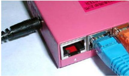
2. Conecte a outra extremidade do cabo à porta LAN
